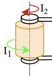
**Fig. 3.1.** The two moments of inertia about Axis-2.
