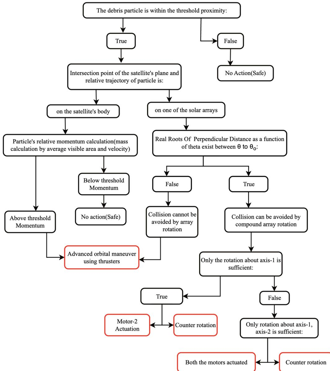
Fig. 7. Flow diagram of the algorithm followed for each individual debris particle.
