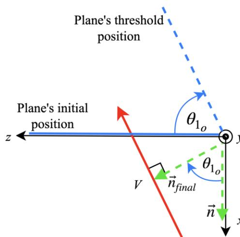
Fig. 6. Top view showing the plane of the satellite, normal vector, and debris particle’s trajectory.
