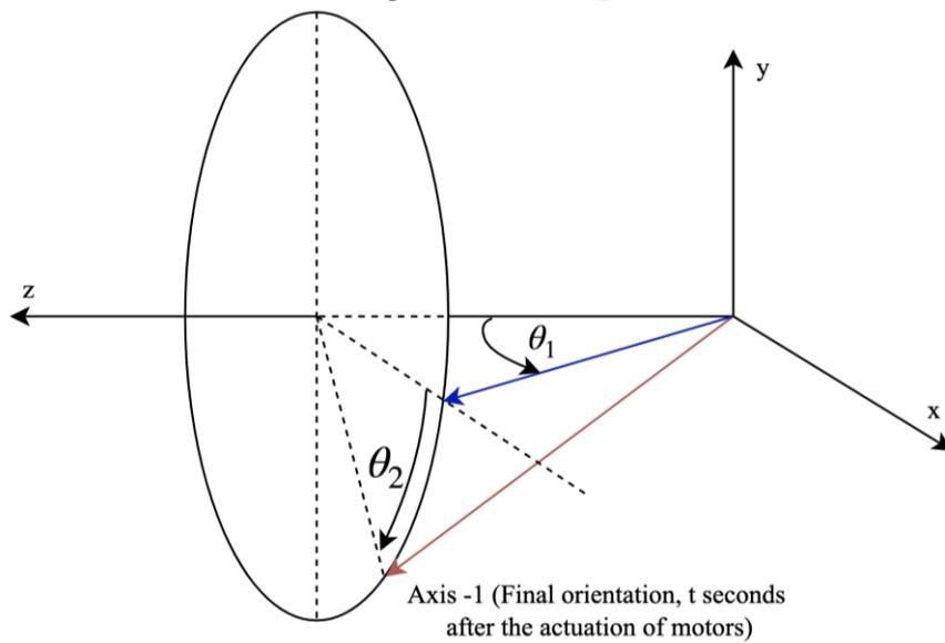
Fig. 2.2.1 Transformation of the Axis1 due to the rotation:  $\theta_2 \rightarrow$  Axis2
