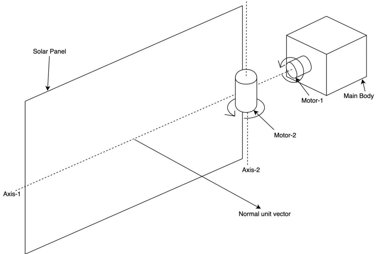
Fig. 1.1 Expanded view of the structure - rigid solar panel's connection to the main body.
