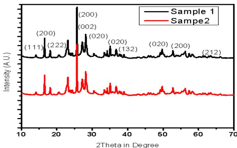
Fig. 1 X-ray diffraction pattern for WO<sub>3</sub> sample 1 and sample 2 at 120<sup>0</sup> C for 12 hours
