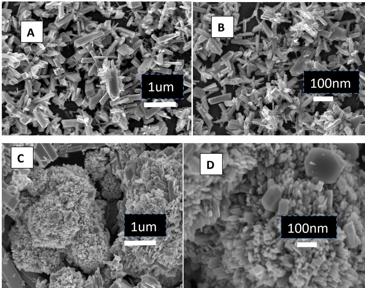
Fig. 2 FESEM image for  $\text{WO}_3$  film Sample 1 (A,B) and Sample 2 (C, D)
