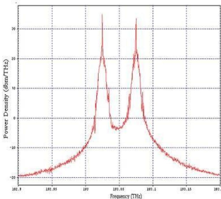
Fig. 2.13: Input Wavelengths (Power density vs. Frequency)
