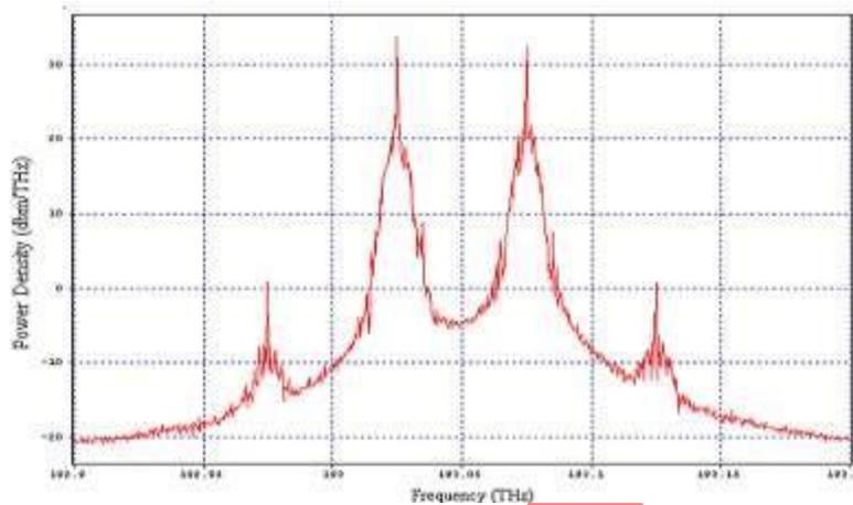
Fig. 2.14: Output Wavelengths (Power density vs. Frequency)
